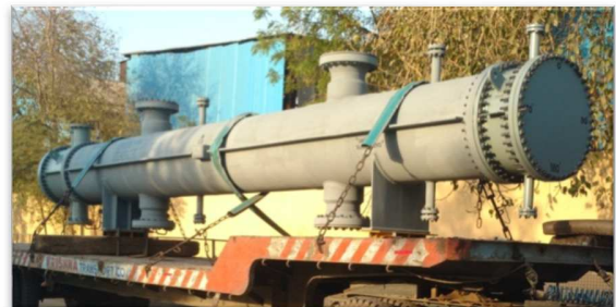
Methanator Effluent Cooler
