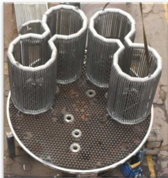
Melamine Reactor Internals
